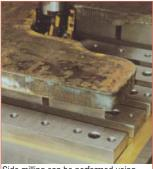
Side milling can be performed using raised blocks for free cutter movement.
